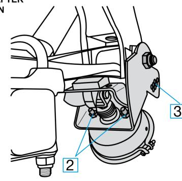
Check M16 Cylinder bolts | 2 | to make sure they are tight. Tighten with a torque wrench if necessary. Tightening torque M16 = 180 - 210 Nm.
